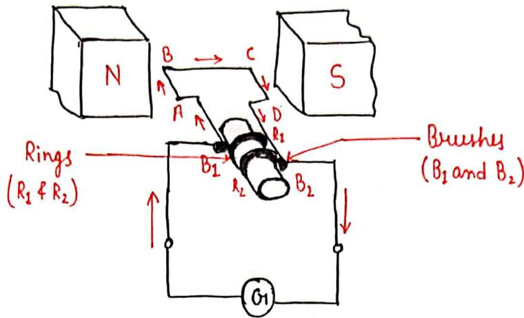
Principle :- It is based on the principle of electromagnetic induction which is the process of producing induced current in a coil by changing its orientation i.e. by rotating it in a uniform magnetic field.
