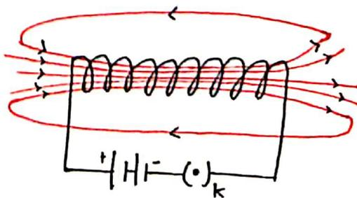
Electromagnet :- It refers to a magnetised solenoid which works on the principle of magnetic effect of current.
