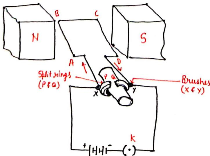
Principle - It works on the principle of magnetic effect of current. When a current carrying conductor is placed perpendicular to the magnetic field, it experiences a force.
